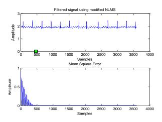
Fig.ure 8. Filtered signal & MSE plot using proposed modified NLMS
