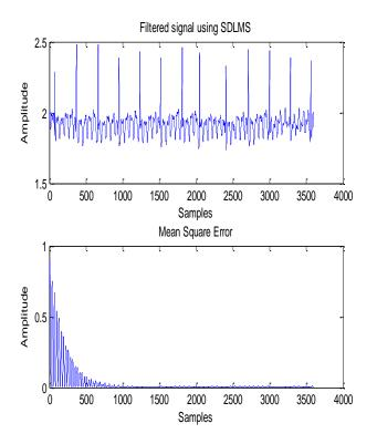
Figure 6. Filtered signal & MSE plot using SDLMS
