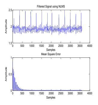
Figure 5. Filtered signal & MSE plot using NLMS
