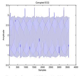
Figure 3. Corrupted ECG signal by PLI type noise
